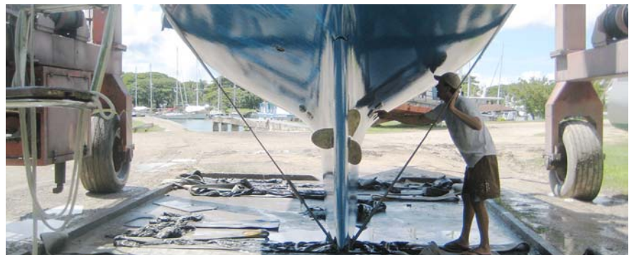
Brian inspects the condition of the zinc on the hull of s/v Skylight while hauled-out for fresh antifouling bottom paint
