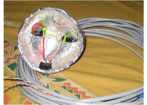
Using parts found around the boat, we turn an old fishing net transponder into LED lighting for the islander's home (a couple of these were made)
