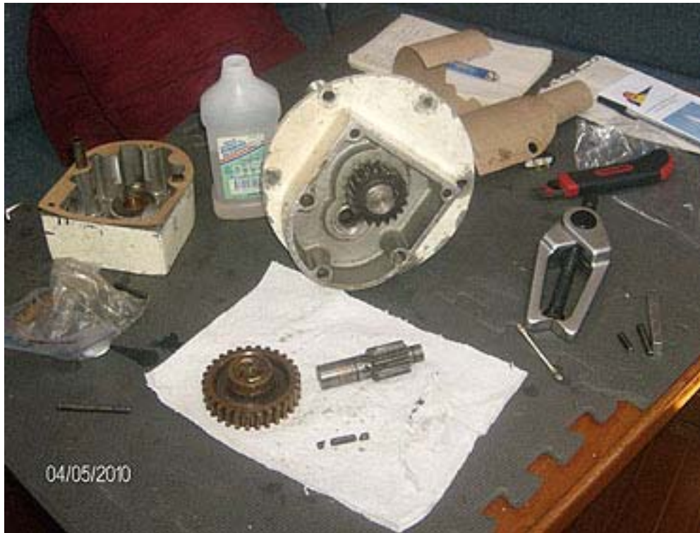
The broken windlass was disassembled, cleaned, repaired, and reinstalled.
